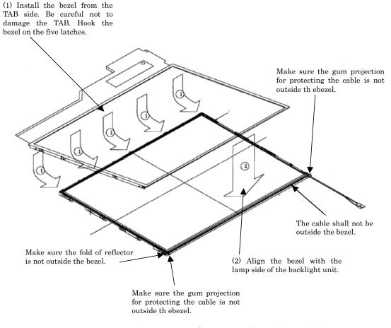
Figure 4-59 Replacing TMD fluorescent lamp (WXGA) (9)
